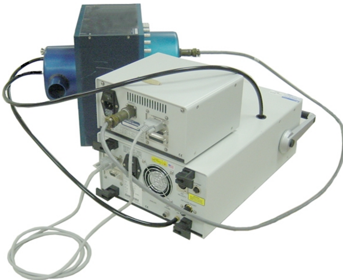
Figure 5. System Connections (power cords not shown for clarity).
